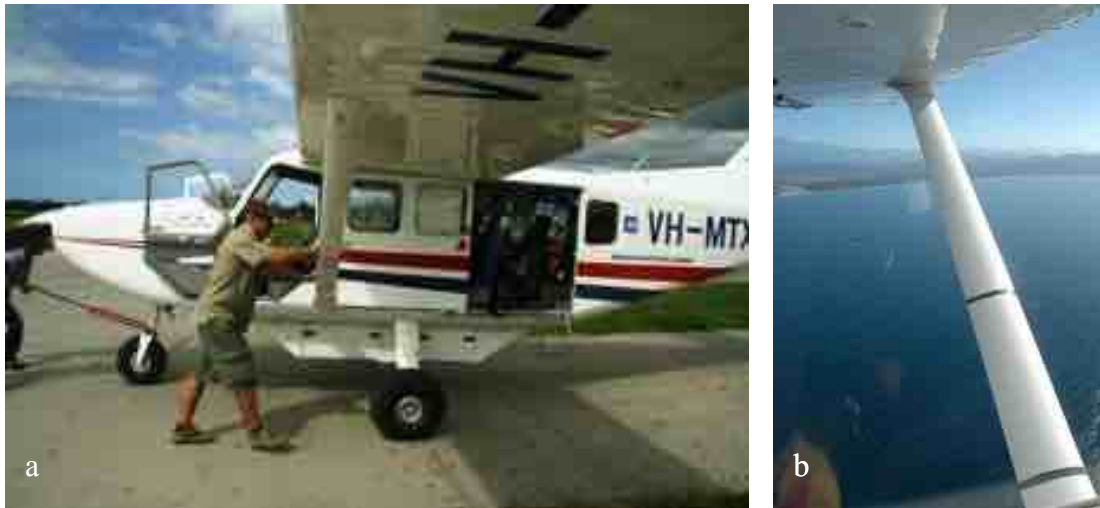
Figure 1. Aircraft used for the aerial surveys (a), and tapes on wing-strut marking the transect width for the observer on the port-side of the aircraft (b).
